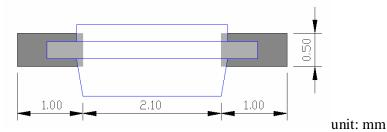
Soldering terminal may shift in x, y direction.
