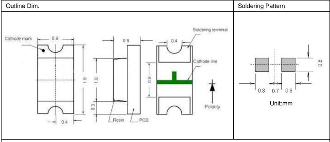
Soldering terminal may shift in x, y direction.
